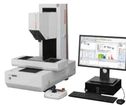
HR-620B PC Interface, Utilizing AVPAK Software
